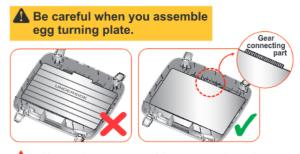
If you do not assemble egg turning place correctly, it can cuase incubator failure.
