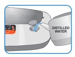
In case you use the incubator without adding humidification water or intend to incubate eggs at low humidity under RH 20%, you must stop its humidification function. please turn off the humidity unit if the unit is empty water otherwise, humidity unit will be broke or you may not no longer use the unit. (When using this function, the alarm for sensing water drop will go out.) [See the description of humidification function OFF on Page 12]
