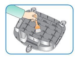
In case the incubator clean status is poor which may cause fan noisy or stopping.
