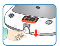
Lock the three locking buttons at the front and rear of the incubator.
